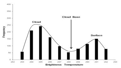
Figure 2: Schematic view of the histogram computed for height assigned.
